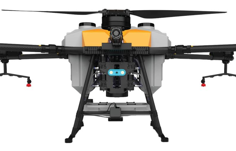
To make the operation more safer, the A-24 Falco comes with a real-time front camera which provides FOV of 120° wide angle. Operators can inspect the real-time condition of where the drone operates. The two LEDs are able to provide better vision for the operators when working at night.
